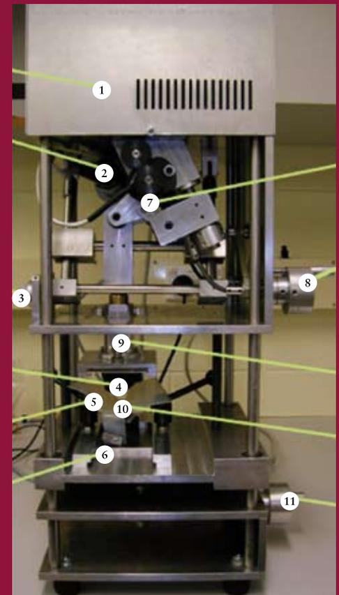
The chewing robot using the 4-bar linkage (above)
